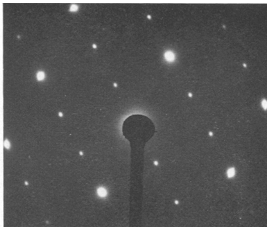
Figure 3 (110)_\beta transmission electron diffraction pattern illustrating the absence of the \omega -phase variants labelled 3 and 4.
