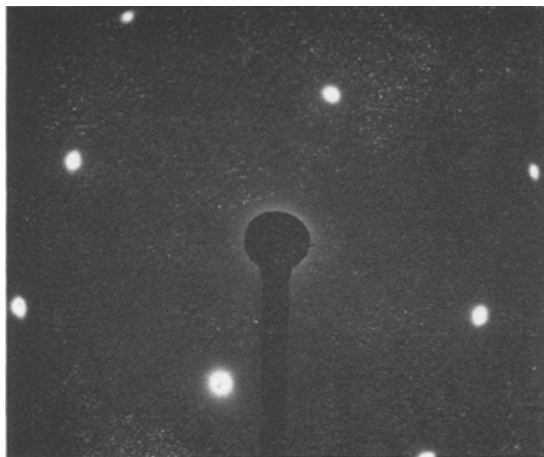
Figure 2 (110)_\beta transmission electron diffraction pattern illustrating the absence of the \omega -phase variant labelled 3.
